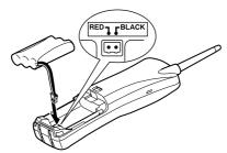
2 Connect the battery pack connector with the correct polarity (black and red wires), then insert the battery pack into the battery compartment.
